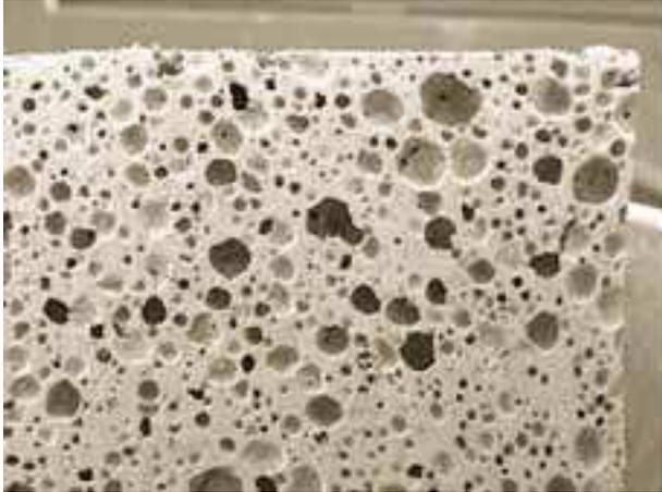
■ Porous structure obtained from foams or sponges used for the filtering of liquids, gases or molten metals; the properties and performance depend on the **ceramic** material chosen. With the most innovative techniques, it is possible to structure the inside walls in a complex way, as shown in the photo on the right, depending on the application requirements. This is the case of catalytic supports which require a very high contact surface for the reactions to take place
